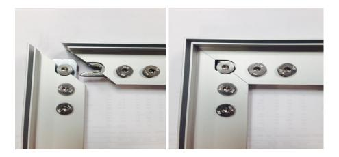
Once the two mitered ends have been put together (note the internal groove that matches with that of the lock), use the supplied 5mm hex wrench to tighten – ensure that the corners come together evenly. <u>CAUTION</u>: the mitered corners are sharp – utilize protective gloves as needed!
