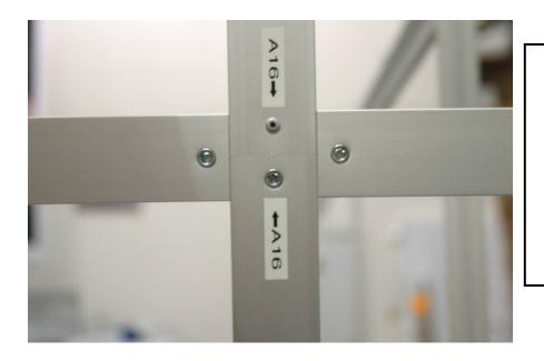
Internal support profiles come together with 3 connections on the frame. Therefore, 3 straight locks form the cross points. Be sure to work these connections while tightening to form good tight connections!
